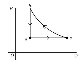
For this gas, Cp = 29.1 J/mol.K. Process ac is a constant pressure process, process ba is at constant volume and process cb is adiabatic. The temperatures of the gas in states a, c and b are  $T_a = 300$ K,  $T_c = 492$ K and  $T_b = 600$ K. Calculate the total work for the cycle. (11 marks)
