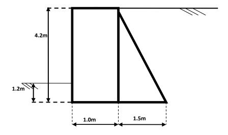
Figure Q1b. Mass concrete Retaining wall
