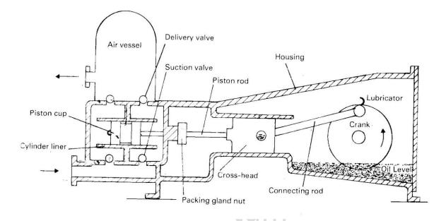
Figure 1: Double – acting piston pump
