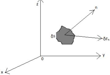
Where  $\delta s$  is a small rigid plane area inserted at a point p in a viscous fluid. The Cartesian coordinates (x, y, z) are a set of fixed axes ox, oy and oz.  $\delta F_n$  is a force exerted by the moving fluid on one side of  $\delta s$ . n Is the unit vector normal at p to  $\delta s$
