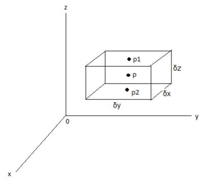
Taking the mass of the fluid element to be constant and the element to move along the fluid. Show that there is a relationship between the Cartesian components
