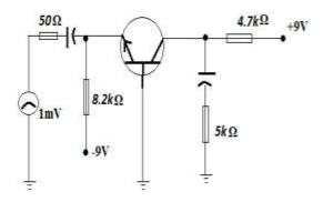
b) If the h-parameter of the transistor were for CE configuration as follows:  $h_{ie} = 1000\Omega$ ;  $h_{re} = -3.5 \times 10^{-4}$ ;  $h_{fe} = 55$  and  $h_{oe} = 20 \mu S$ . Find the current gain,  $A_i$  and voltage gain,  $A_v$  if  $r_L$  $=2k\Omega$ . (8mks)
