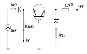
b) If the h-parameter of the transistor were for CE configuration as follows:  $h_{ie} = 1000\Omega$ ;  $h_{re} = -3.5 \times 10^{-4}$ ;  $h_{fe} = 55$  and  $h_{oe} = 20 \mu S$ . Find the current gain,  $A_i$  and voltage gain,  $A_v$  if  $r_L$  $=2k\Omega$ . (8mks)
