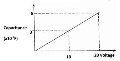
Use the graph to determine the quantity of charge stored in the capacitor.
