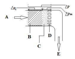
(e) Given the following cross section of a centrifuge, and that  $dF_c = (dm)r\omega^2$  while  $dP = \rho\omega^2 rdr$ , derive the equation for the determination of neutral radius (9 Marks)
