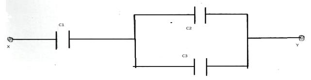
If C1=  $6\mu$ F, C2= $4.5\mu$ F and C3 =  $7.5\mu$ F. Calculate the effective capacitance. (4mks)
