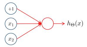
Given the parameter values as -30, 20,20, respectively, determine the output of the hypothesis.
