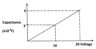
Use the graph to determine the quantity of charge stored in the capacitor.
