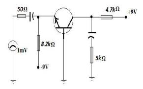
b) If the h-parameter of the transistor were for CE configuration as follows:  $h_{ie} = 1000\Omega$ ;  $h_{re} = -3.5 \times 10^{-4}$ ;  $h_{fe} = 55$  and  $h_{oe} = 20 \sim S$ . Find the current gain,  $A_i$  and voltage gain,  $A_v$  if  $r_L = 2k$ . (8mks)
