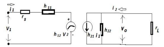
Given that the sketch is a reduced CE amplifier connection network with a quiescent current of 1mA having manufacture specifications as  $h_{11} = 3.5k$ ;  $h_{12} = 1.3 \times 10^{-4}$ ;  $h_{21} = 120$ ;  $h_{22} = 85\mu S$  and  $r_s = 1k$ .
