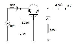
b) If the h-parameter of the transistor were for CE configuration as follows:  $h_{ie} = 1000\Omega$ ;  $h_{re} = -3.5 \times 10^{-4}$ ;  $h_{fe} = 55$  and  $h_{oe} = 20 \sim S$ . Find the current gain,  $A_i$  and voltage gain,  $A_v$  if  $r_L$ =2k . (8mks)
